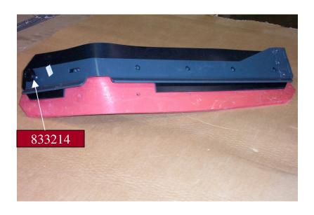
CLOSE WELD-RETAINER RH (3333202) OVER THE SQUEEGEE BLADES. (MAKE SURE THE PINS ARE CENTERED IN THE HOLES. TIGHTEN SCREWS WITH ½ INCH WRENCH. ATTACH KNOB-3 SIDED (833214).
