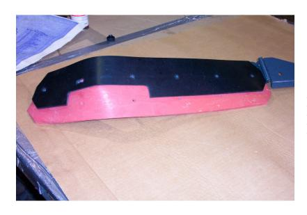
ATTACH STIFFNER-SQUEEGEE BLADE (333166) TO WELD SQUEEGEE BLADE RH (3333131).
