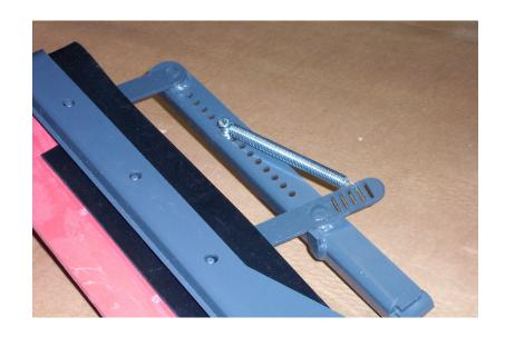
ATTACH SPRING-EXTENSION SIDE SQUEEGEE (333167) TO WELD ARM (333138) AND WELD-SQUEEGEE ARM (333084). SECURE WITH SCR-HEX,1/4-20X0.88 ZP (3400041) AND 2EA. NUT-FLANGE LOCK 1/4-20 ZP (3400063).
