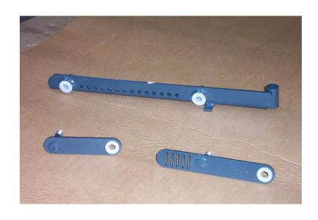
ATTACH 2EA. BUSHING-3/8 NYLON (3333105) TO WELD-SQEEGEE ARM RH (333084). ATTACH 1EA. BUSHING-NYLON 3/8 TO WELD-ARM (333139) AND 1EA. BUSHING-NYLON 3/8 TO WELD-ARM (333138).
